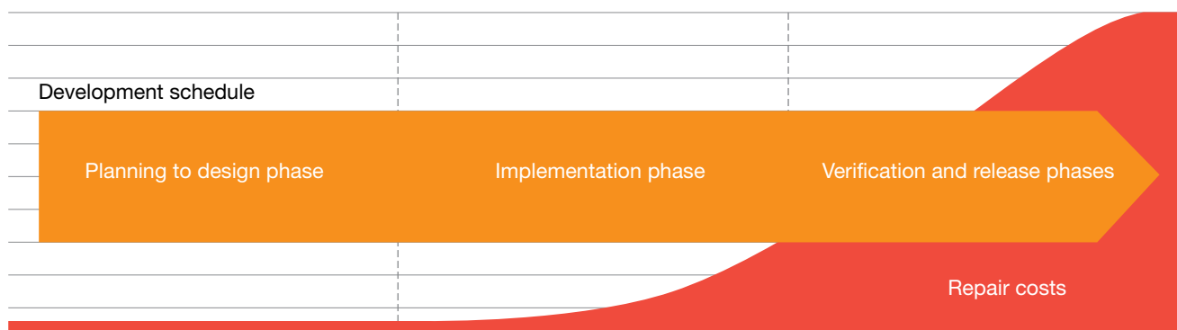
Diagram 19: Repair costs that rise in conjunction with the progress of development process
